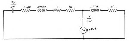
Fig. 10-Simplified circuit diagram of moving coil microphone at low frequencies.
