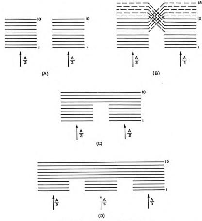
Fig. 6-Genesis of a graded multiple.
