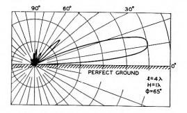
Fig. 17-Vertical plane directive diagram.
