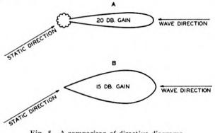
Fig. 5-A comparison of directive diagrams.
