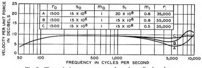
Fig. 7-Theoretical response curves of moving coil microphone.
