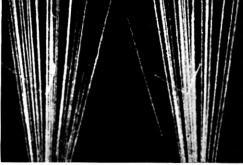
Fig. 10—Transmutation of a nitrogen atom attended by capture of the impinging alpha-particle (P. S. Blackett).
