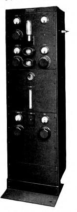
Fig. 3-Front view of crystal controlled oscillator-amplifier unit.
