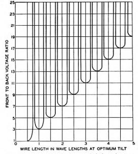
Fig. 13-Front-to-back ratios for characteristic impedance termination.
