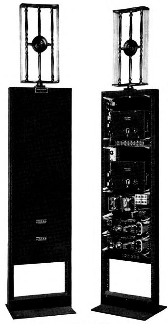
Fig. 7—Remote controlled monitoring point receivers. Fig. 8—Can covers removed from rear of monitoring point receivers to show the location of the receivers and remote control relays.
