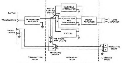
Fig. 1-Schematic circuit diagram of essential apparatus.
