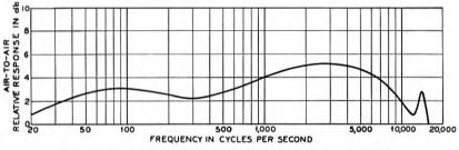
Fig. 3-Reproduction-ratio characteristic of complete system.
