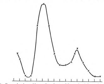
Fig. 4—Curve showing evidence that the particles emitted from aluminium bombarded by  $\alpha$ -rays comprise protons and deflected alpha-particles (G. Stetter).
