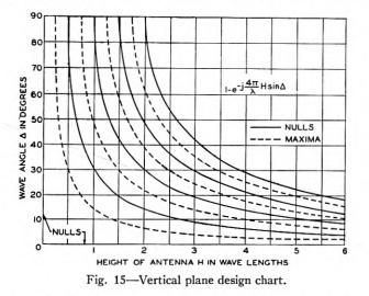
detail a sample of the design methods employed and the performance measurements on one typical form of antenna; accordingly a medium size horizontal diamond-shaped antenna has been selected.
