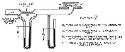
Fig. 5-Method used to measure acoustic resistance.
