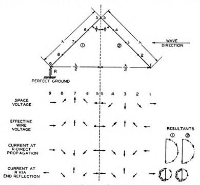
Fig. 10-Vector relations in an inverted V antenna.
