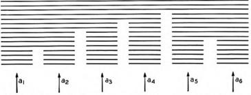
Fig. 7(B)—Example of a non-symmetrical progressive graded multiple.
