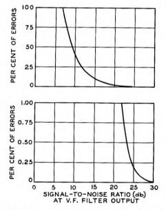
Fig. 5—Relation between printer errors and signal-to-noise ratio as determined from the Rocky Point-to-Rochester tests.
