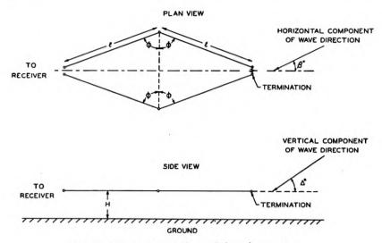
Fig. 14-The horizontal diamond-shaped antenna.
