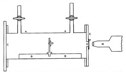
\* Fig. 1—Rutherford's apparatus for detecting transmutation of gases by the scintillation method. Source of alpha-particles at D; gas in the tube; fluorescent screen (transparent) at S; microscope at M.
