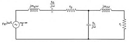
Fig. 2-Circuit diagram for receiver or microphone.
