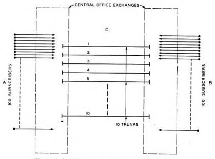
Fig. 2-A simplified central office interconnection system.
