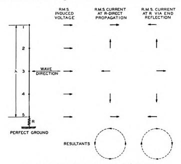
Fig. 7-Vector relations in a one-wave vertical antenna.
