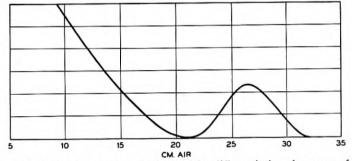
Fig. 9—Distribution-in-range curve obtained by differentiating the curve of Fig. 8 for boron (W. Bothe and H. Fränz).
