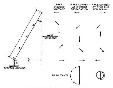
Fig. 8-Vector relations in a tilted wire antenna.
