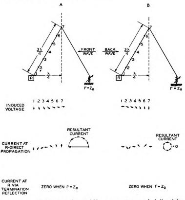
Fig. 11-Vector relations in an inverted V antenna-asymmetrical directivity.
