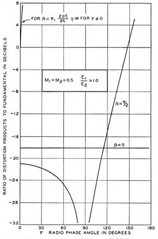
Fig. 15—Ratio of distortion products to fundamental with 50 per cent modulation of each carrier for varying audio and radio phase angles,  $\beta$  and  $\gamma$  respectively, where the field strength ratio  $E_1/E_2 = 1$ .
