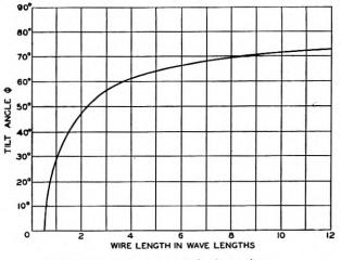
Fig. 9-Optimum tilt angle for long wires.
