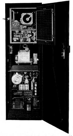
Fig. 4-Rear view showing interior of oscillator-amplifier unit.
