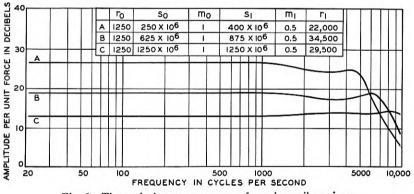
Fig. 3-Theoretical response curves of moving coil receiver.
