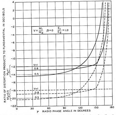
Fig. 12—Ratio of distortion products to fundamental for the point directly between and equidistant from the two stations, with varying carrier phase angle,  $\gamma$ , and different degrees of modulation of the two carriers,  $(V = M_1/M_2)$ , where the audio phase angle  $\beta = 0$  and the field strength ratio  $E_1/E_2 = 1$ .
