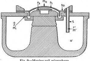
Fig. 9-Moving coil microphone.
