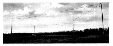
Fig. 22-An experimental horizontal diamond-shaped antenna.
