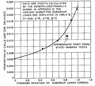
Fig. 21-Effect of subgroup load variation on probability of loss-52 graded trunks.
