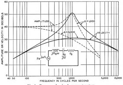
Fig. 1-Response of a simple resonant system.
