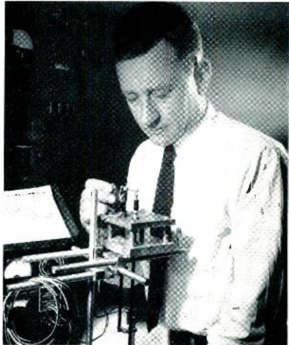
*J. J. Forst adjusting an ultra-sensitive semiconductor strain gauge constructed with germanium.*
