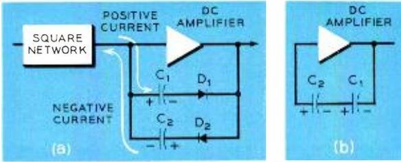
(a) Amplifier circuit to compute average square of its input voltage. Capacitors are connected in series with oppositely poled diodes  $D_1$  and  $D_2$ .
