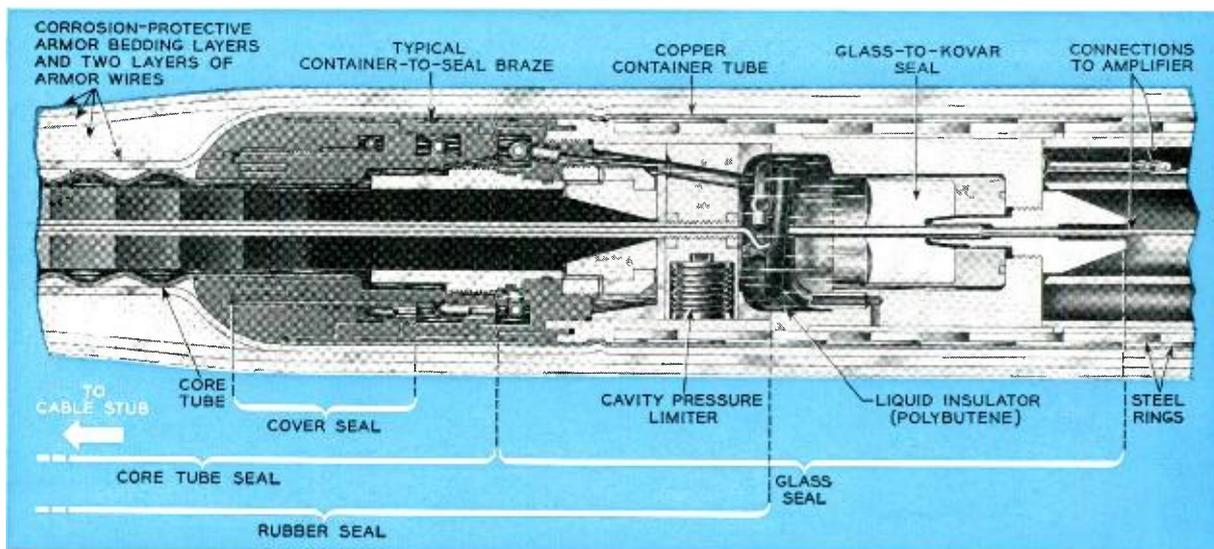
*Internal construction of an undersea telephone cable repeater. Repeater enclosure is terminated at each end with a system of seals: glass-metal,*
