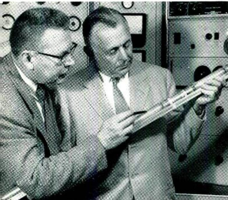
*W. A. Klute (left) and W. M. Bishop examine an amplifier section. This view shows the unsheathed amplifier with adjacent sections attached to each other; they are connected electrically by bus tapes.*
