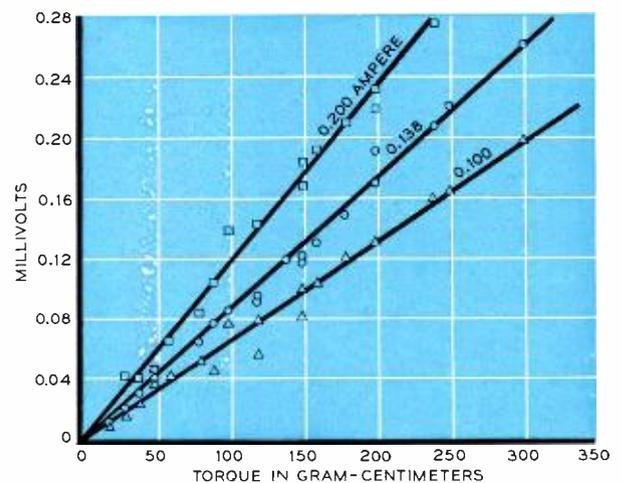
Configuration of the torsional transducer. Graph shows calibrations at different biasing currents.
