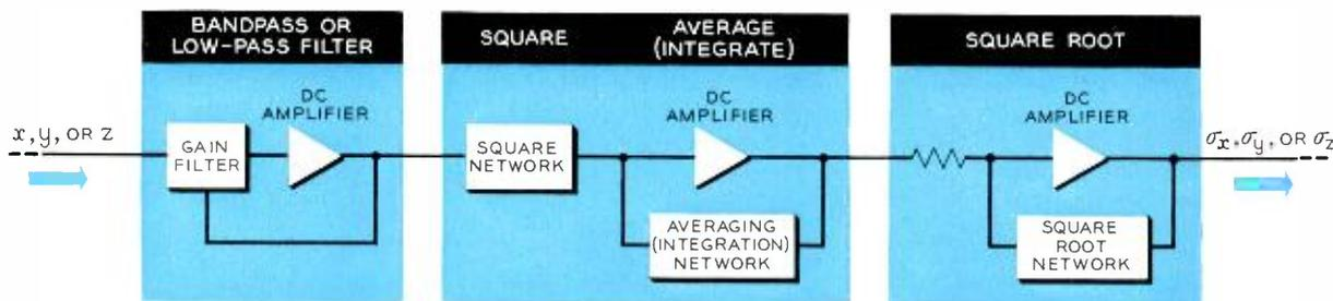
*Simplified schematic showing the three dc amplifiers that (left to right): filter incoming wave-*
