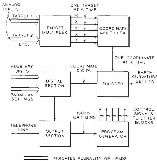
Fig. 3 — Block diagram of AN/TSQ-7 transmitter.
