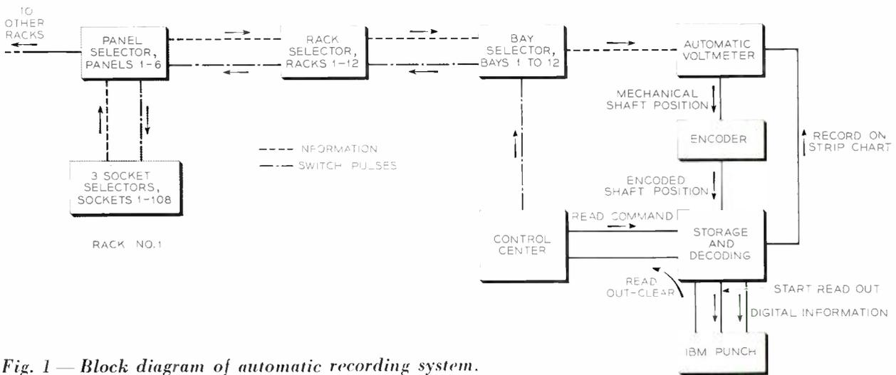
Fig. 1 — Block diagram of automatic recording system.
