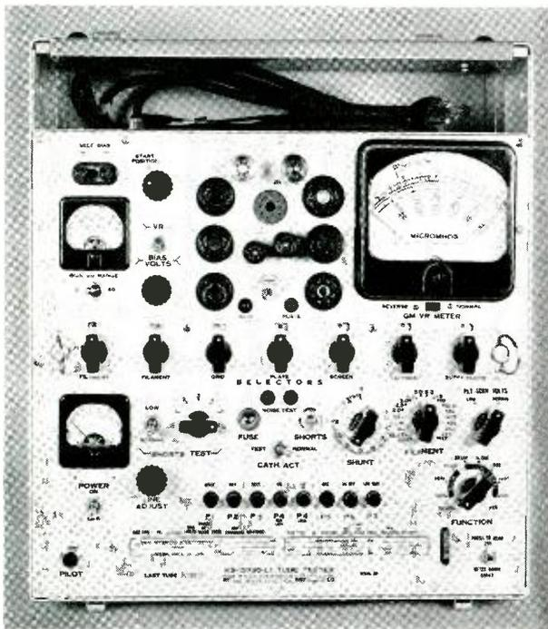
Fig. 1 — Front panel of the improved tube tester.
