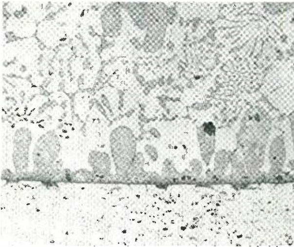
Fig. 2 — Photomicrograph of a joint showing complete wetting of the aluminum (bottom) by the zinc-base solder (top). Original magnification 500x.
