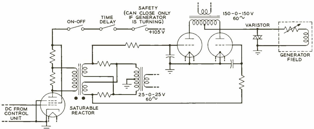
Fig. 7—Schematic circuit of field current supply.
