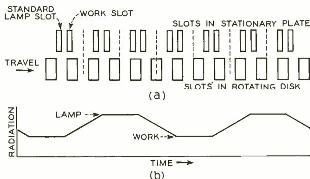
Fig. 2—Optical commutation cycle.
