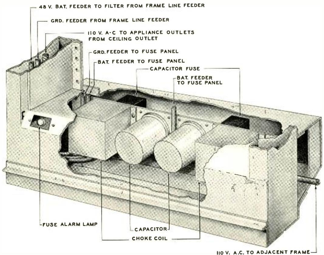
Fig. 6—Perspective drawing showing arrangement of base of the No. 5 crossbar frame.
