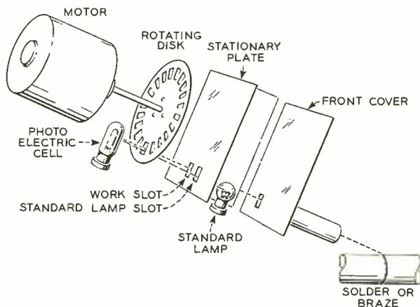
Fig. 1—Optical commutator for temperature control.
