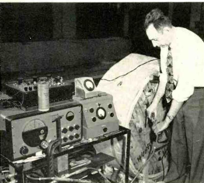
*R. A. Kempf is preparing a test arrangement to make measurements on a reel of coaxial cable under varying temperature conditions.*
