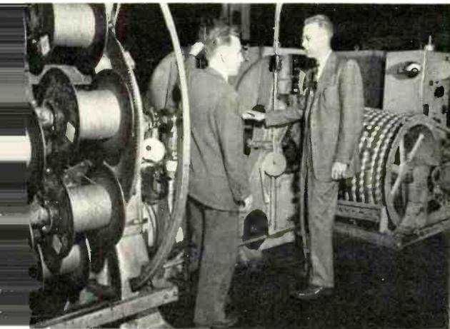
*N. V. Firth (center) and E. V. Rice (Western Electric) (right) are checking the wire armoring of lead covered cable as it passes through the armoring machine. Operator of the machine is J. M. Seglinski, Western Electric.*
