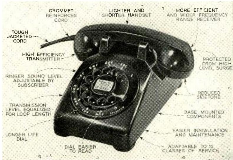
of the war that if a completely new set could be developed as an integrated unit, taking full advantage of improvements in structures, materials and design techniques, as related to service requirements, it would be possible to provide a new telephone set that would be still better than the 302. The development was started; the new set was ready for its first field trials by 1948, was placed in limited production in 1949, and production has been steadily increasing since then.
