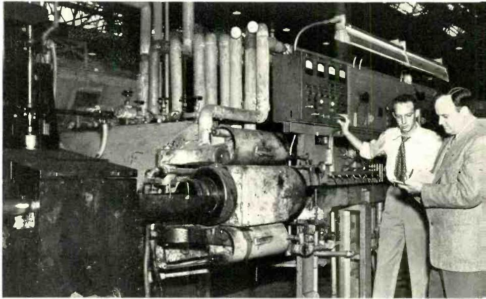
*C. R. Noble (right) with E. D. Long (Western Electric) review the operation of the plastics extrusion machine for applying the polyethylene jacket to a Lepeth sheathed cable core. The cable core enters the extrusion die at the left, and the covered core emerges from the die to enter the water trough just below Mr. Long's right arm.*
