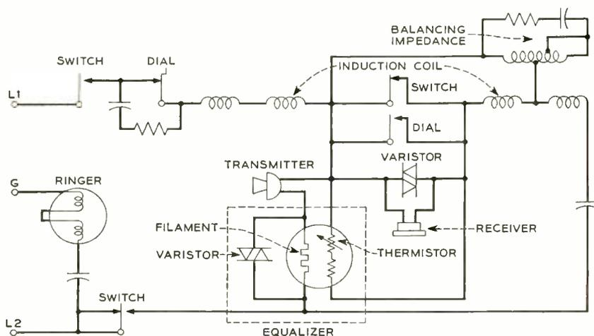
Fig. 2—Schematic of 500 type telephone set.
