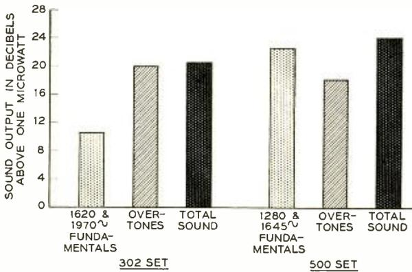
Fig. 6—Ringer sound output spectrum.
