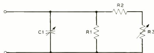
Fig. 5—Balancing network.
