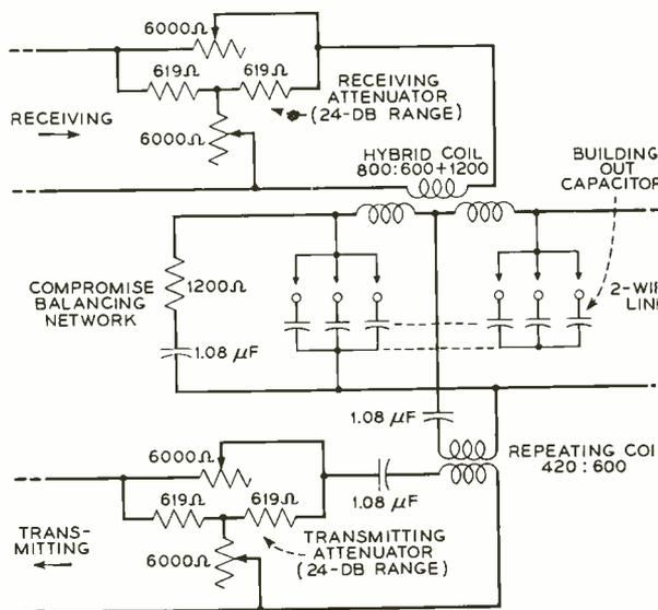
Fig. 1—Schematic of the new miniature four-wire terminating set.
