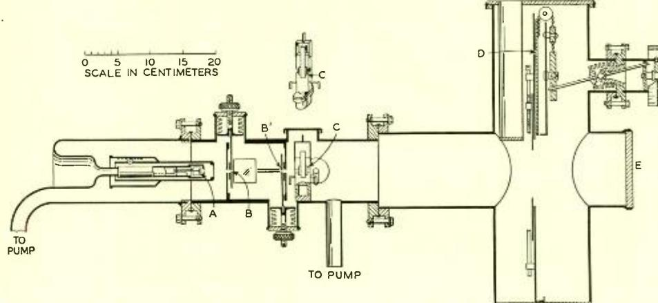
*Fig. 4—Longitudinal cross-section of the electron diffraction camera*
