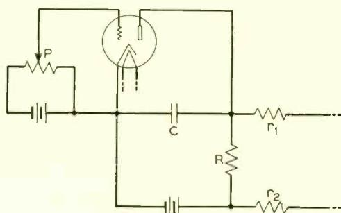
Fig. 1—A gas tube relaxation oscillator, shown here diagrammatically, is used to provide a rapid succession of timed pulses
