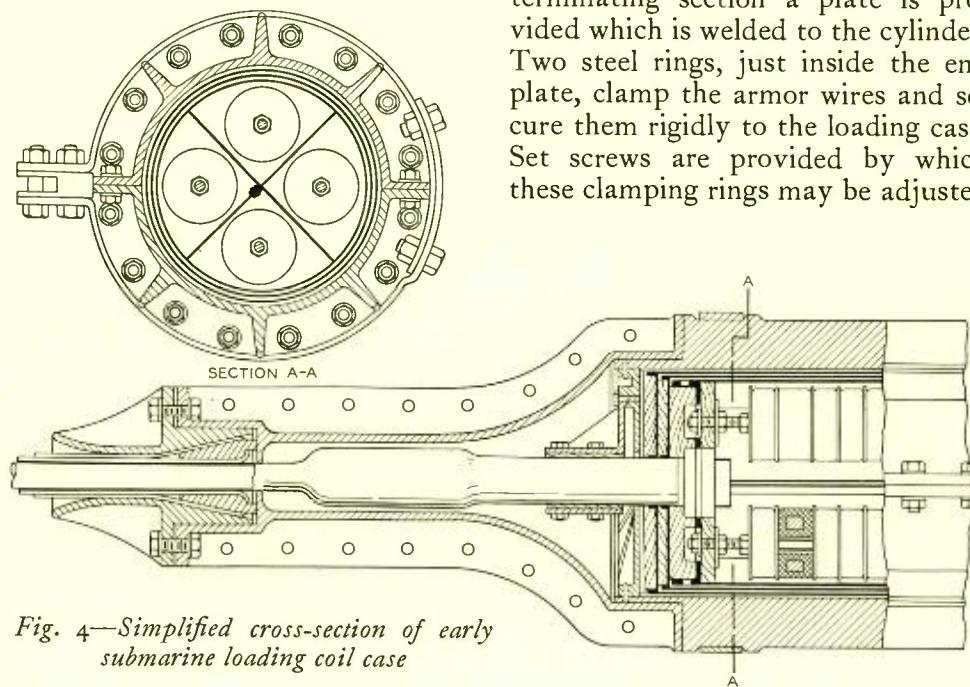
*Fig. 4—Simplified cross-section of early submarine loading coil case*
