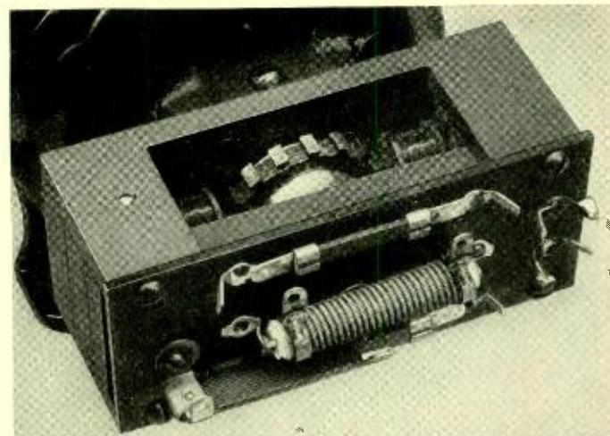
*Fig. 2—Between the inductor coils, which are mounted in a rectangular structure on the end of the inductor-alternator, is a laminated iron rotor with seventeen teeth*
