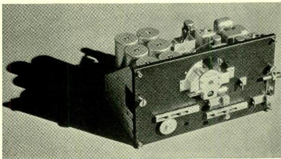
*Western Electric 20-type radio receiver developed by the Laboratories to provide a light, compact set of extreme selectivity for use in small aircraft. The receiver is designed for either remote (shown above) or local control and is provided with four frequency bands covering a range from 200 kilocycles to 10,000 kilocycles*
