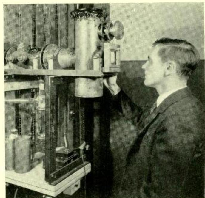
*Fig. 1—K. H. Storks of the Research Department adjusting the camera preparatory to making a photographic record of an electron diffraction pattern*
