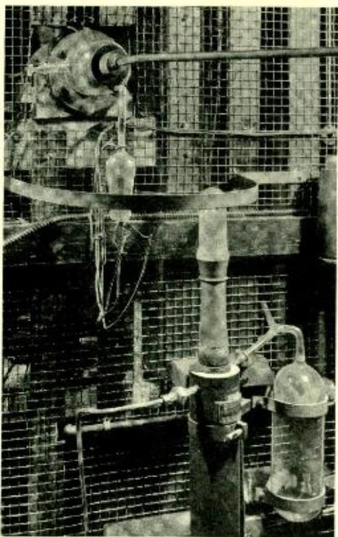
*Fig. 2—The filament end of the camera. The filament is maintained at a potential of 50 or 60 kilovolts negative to ground. The transformer, rectifier, and filter which supply the high negative potential to the filament are shown in the headpiece*
