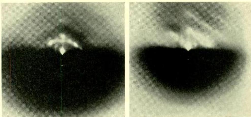
*Fig. 3—Diffraction patterns from oriented layers of stearic acid molecules*
