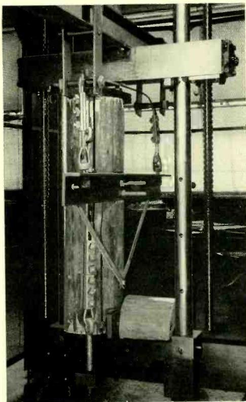
Fig. 2—The strengths of steel crossarms and attaching bolts are determined by mounting them on a pole section in the Amsler machine. The braces are removed before testing
