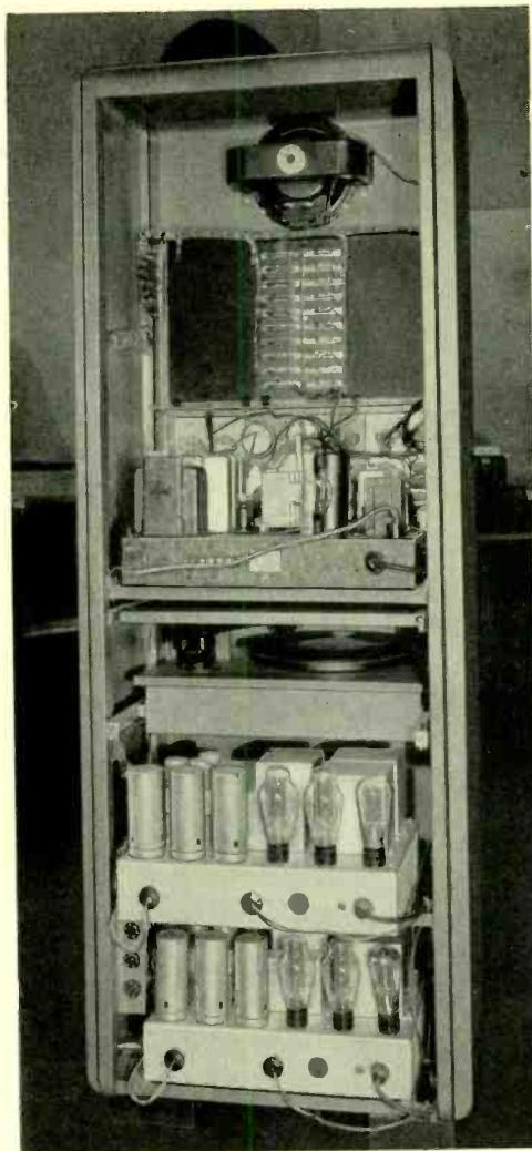
Fig. 2—The two amplifiers, and radio set are mounted on shelves which slide out from the back of the cabinet for adjustments
