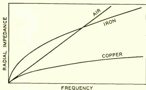
*Fig. 1—Radial impedance of all materials increases with frequency: the graph for air and other dielectrics is a straight line; the graphs for magnetic materials, of which only one is shown, are curves which have values greater than those of air for lower frequencies, and less for higher frequencies. The radial impedance of copper and other non-magnetic materials is always less than the value found for air*
