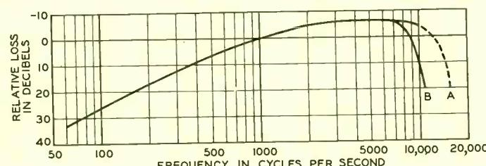
Fig. 1—Frequency weighting curve for program circuit noise. Curve A for circuits transmitting all audible frequencies up to fifteen thousand cycles and Curve B for those cutting off at eight thousand cycles
