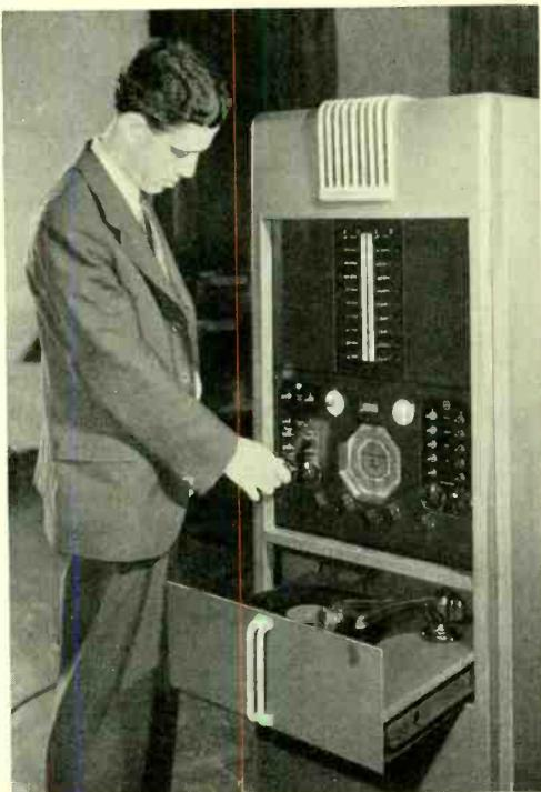
Fig. 1—The new program sound system comprises a radio receiver, a phonograph and three microphone input circuits
