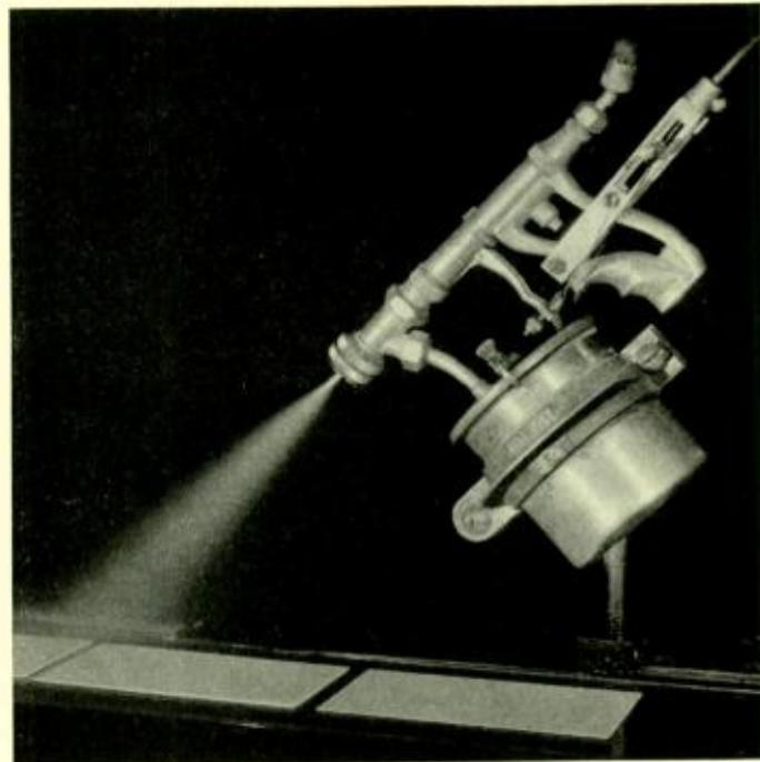
*Fig. 2—Several panels can be sprayed simultaneously*
