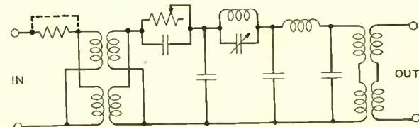
Fig. 3—Circuit schematic of frequency-weighting network for program circuit noise measurement
