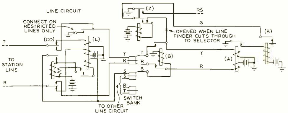
Fig. 3—For larger PBX's using the 200-point line finder, a special arrangement using relay Z is required to obtain restricted service
