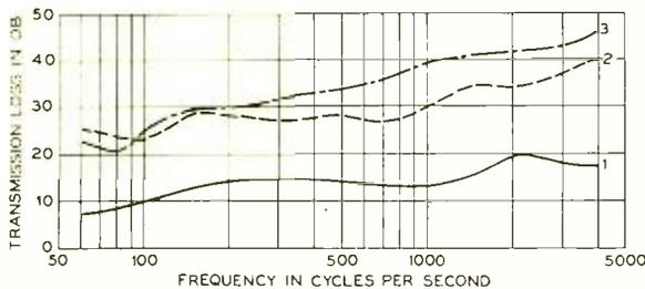
*Fig. 3—Typical transmission-loss curves for various types of walls*
