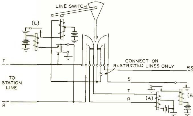
Fig. 2—With private branch exchanges using the line switch a fourth wire is available to serve as the RS lead
