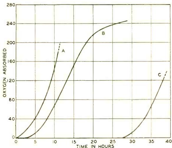
Fig. 4—These curves show that the oxidation of hydrocarbon oil at  $120^{\circ} C$  occurs sooner in the presence of the positive catalyst, copper (A), than alone (B), and can be greatly delayed by as little as .01% of a negative catalyst or antioxidant (C). The absorbed oxygen is expressed in cubic centimeters per gram of oil
