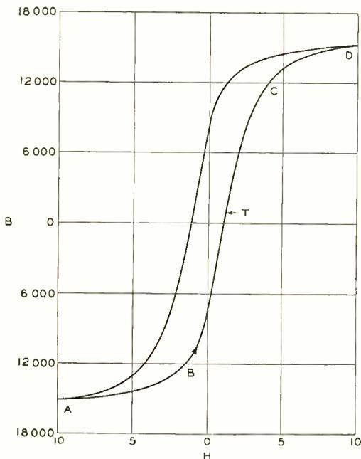
Fig. 2—An ordinary magnetization curve of iron
