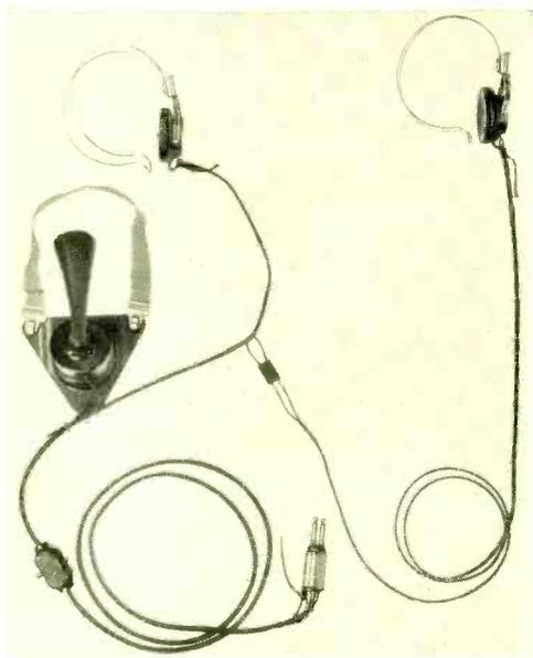
*Fig. 2—A supervisor's cord showing connecting block from chief operator's headset*
