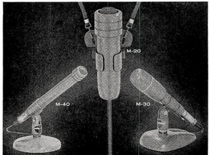
M-40 response 40-20,000 cps • output -57 db • 9½ inches long, 1 inch in diameter • 17 ounces. M-30 response 50-18,000 cps. • output -57 db • 6½ inches long, 1¼ inches in diameter at head • 16 ounces. M-20 response 60-18,000 cps • output -57 db • 4 inches long, 1 inch in diameter • 3½ ounces. For more information contact your Collins sales engineer or write.
