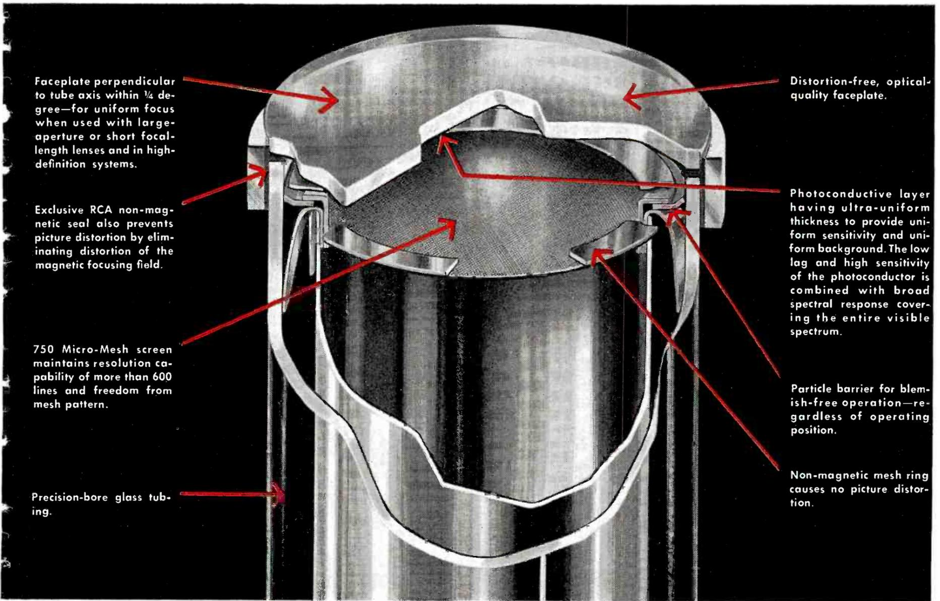
Faceplate perpendicular to tube axis within 1/4 degree—for uniform focus when used with large-aperture or short focal-length lenses and in high-definition systems.
