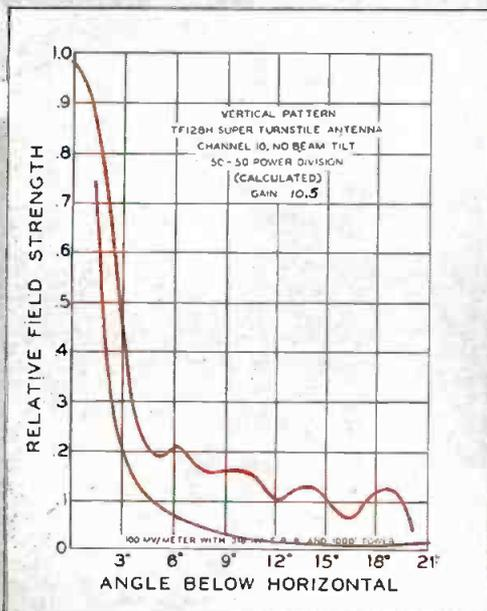
**Vertical Field Pattern of new RCA TF-12BH 50-kw antenna.** Note complete absence of vertical nulls. Operated in conjunction with an RCA 50-kw TT-50AH transmitter, this antenna will "saturate" your service area with strong signals.
