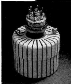
*GL-8002-R's radiator is milled from solid copper. Air passages are of uniform width for more efficient cooling. Total height, including radiator, is 5 3-8 inches; total diameter, 3 11-16 inches.*
