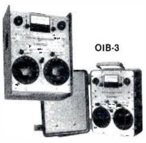
The Operating Impedance Bridge measures the impedance of networks, radiators, and the like while they operate under full power. VSWR as well as complex impedances of up to 400  $\pm$  j300 ohms can be measured.
