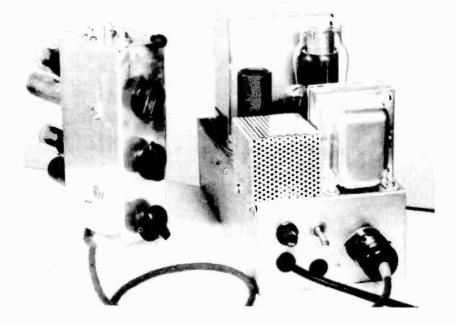
Fig. 1. Compact, two section amplifier with control section arranged for mounting in small panel area.
