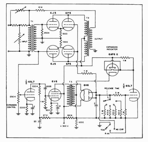
Fig. 1. Schematic diagram of the high-fidelity volume expander.
