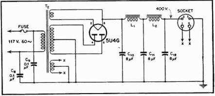
Fig. 3. Schematic of the power supply.
