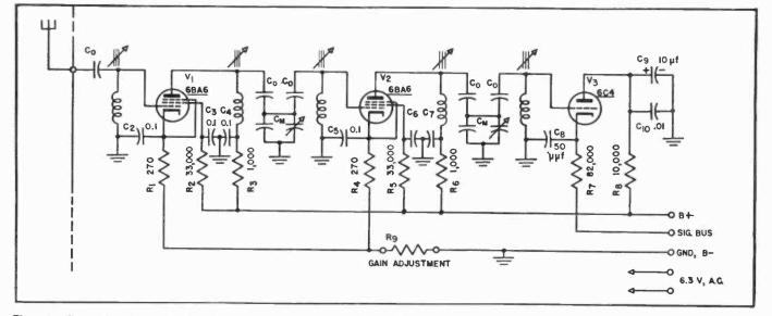
Fig. 10. Over-all schematic for the AM tuner strip. Values for Co and Cw are given in the text. Table I, and Fig. 11.
