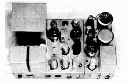
Fig. 23. Top view of the main amplifier and power supply units bolted together as a single chassis.
