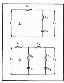
Fig. 3. (A) Single-section RC network used to provide low frequency boost at the rate of 3 db/octave. (B) Two sections are necessary for a boost of 6 db/octave.
