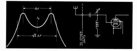
Fig. 7. (left). Curve resulting from over-coupled circuits of Fig. 6. The usable band width is represented by the limits √2 △f. The valley between the peaks can be filled by using a single-tuned circuit in conjunction with the doubletuned circuits. Fig. 8. (right). Method of coupling the antenna to each of the tuner strips. This enables tuning the antenna circuit for each station and provides adequate signal input to the first stage.
