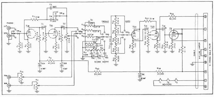
Fig. 5. Schematic of the control section.
