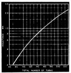
Fig. 7. Chart for determining number of turns to give inductance values necessary for various networks. This chart applies to coils wound on 11/4" core of wooden spool to a width of 3/4", using #16 enameled wire with 13 turns per layer.
