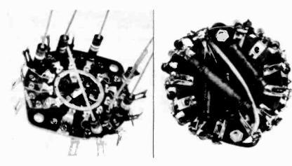
Fig. 5 (left). First step in connecting the resistors to the 1443 switch deck. The 0.15-meg shunt resistors are mounted first, as shown. Fig. 6 (right). Method of mounting the compensating capacitors on the de-rotored "B" switch deck.
