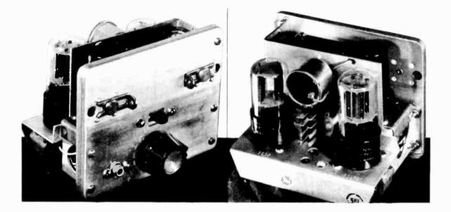
Fig. I. Equalizer-suppressor amplifier as built on surplus preamplifier chassis.
