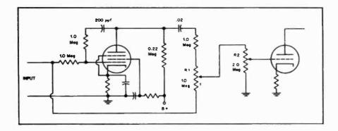
A single-tube amplifier circuit claimed to furnish sufficient equalization for magnetic phonograph pickups together with an appreciable amount of amplification is described by J. Ellis in Wireless World for September, 1947. The circuit, shown at left employs a single pentode with feedback to provide the desired frequency response.
