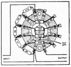
Fig. 26. Method of constructing input attenuator on a single switch deck. The contact fingers on one half are bent back or cut off, and the lugs serve only to mount the resistors.
