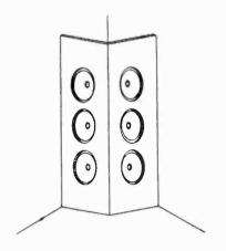
Fig. 1. Mounting a number of ordinary cones on two sides of an obtuse structure for corner use is one solution to the necessity for moving more air.
