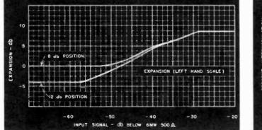
Fig. 4. Input signal level vs. expansion curves.
