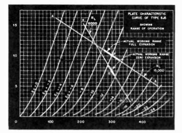
Fig. 2. Curves showing operating range of expander tubes.
