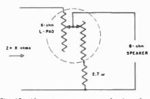
Fig. 15. Alternate arrangement showing the use of a 6-ohm L-pad in an 8-ohm circuit to provide a maximum loss of 12 db.
