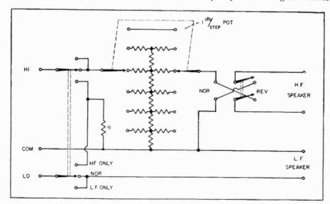
Fig. 7. Test unit for simplifying the balancing and phasing of I-f and h-f speakers.
