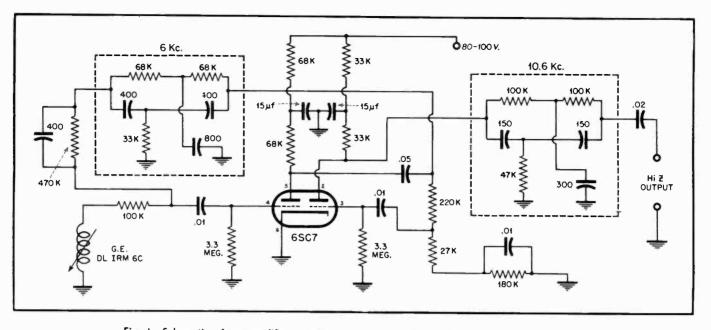
Fig. 1. Schematic of pre-amplifier and filter circuit especially suited for magnetic pickups.
