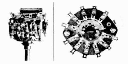
Fig. 1A (left). The fully compensated volume control assembled on a Centralab 1443 switch. Fig. 1B (right). The decompensator made from a modified "G" switch deck and mounted on a standard index assembly.
