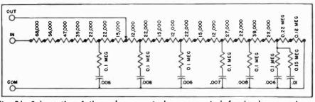
Fig. 21. Schematic of the volume control compensated for loudness contours.
