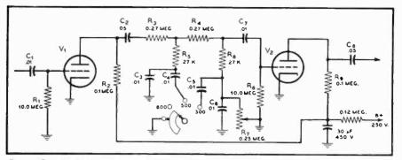
Fig. 1. Equalized two-stage amplifier suitable for low-frequency compensation for modern high-quality, low-level magnetic pickup cartridges.
