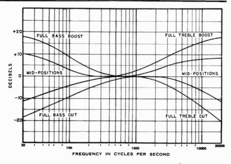
Fig. 5. Characteristics of dual tone control.
