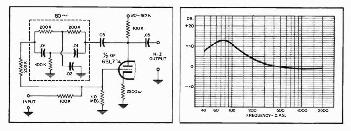
Fig. 3 (left). Circuit to provide bass boost, and Fig. 4 (right), its response curve.
