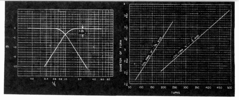
Fig. 2 (left). Frequency-response characteristics of dividing network of Fig. 1. Fig. 4 (right). Flange diameter required for coil forms for coils having given number of turns of No. 17 DCE wire.
