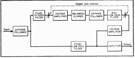
Fig. 2. Second experimental circuit, incorporating fewer filters.
