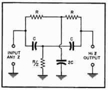
Fig. 5. Fundamental filter circuit.
