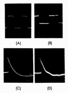
Fig. 6. Oscillograms of output for various input signals: (A) 200-cps square wave; (B) 5000-cps square wave; (C) 0.5-volt d-c pulse at input, speaker connected normally; (D) same signal as at (C), but with 10-ohm resistor in series with voice coil. Last two oscillograms show effect of damping.
