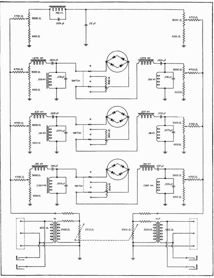
Fig. 5. Complete schematic of the experimental noise suppressor.
