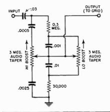
The network is shown at left and the values shown give substantially the same response curves as shown in the article. The input should be connected to a source impedance not higher than about 20,000 ohms, to prevent loss at high frequencies when in the high boost position, and the output should work directly into a grid, as pointed out in the editorial note.
