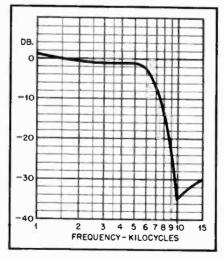
Fig. 2. Reponse curve of amplifier and filter shown in Fig. 1.
