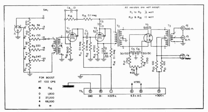
Fig. 24. Schematic of the main amplifier, closely following the original 6AS7G amplifier described back on page 5.
