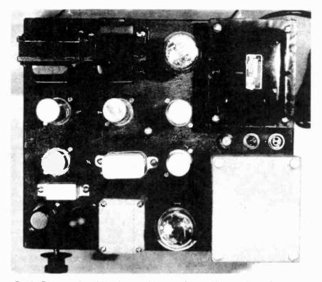
Fig. 3. Top view of amplifier, showing placement of parts. Note simplicity of arrangement. Capacitor above interstage transformer is C4, used in shunt feed circuit. Note use of inverted can capacitor for coupling between 6SJ7 and 6N7, shown directly above the two tubes.
