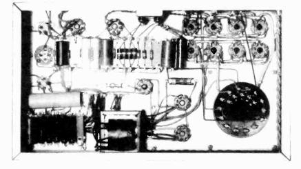
Fig. 2. Underside of amplifier chassis. Note clean, straightforward wiring layout.
