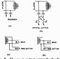
Fig. 7. Change in output wiring for feeding different types of recorders.
