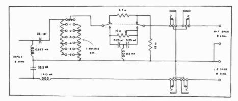
Fig. 17 Complete circuit of dividing network, h-f attenuator, 10-kc suppressor, and jacks to permit access to the various circuits.
