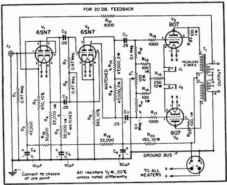
Fig. 2. Schematic of the amplifier section.
