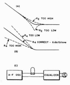
Fig. 17. Phonograph equalization curves at A and B show the effect of resistor values. C shows method of connecting oscillator to obtain correct results.
