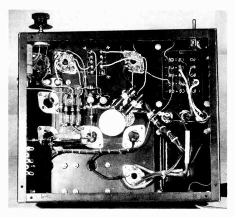
Fig. 4. Under-chassis view of amplifier.
