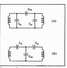
Fig. 6. Two methods of obtaining band-pass coupling by the use of two tuned circuits and an impedance common to both. (A). High-impedance capacitance coupling; (B). Low-impedance capacitance coupling
