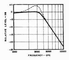
Fig. 3. Shape of response curve for  $f_{\rm c}=3850$  cps. Dotted curve indicates peak due to improper terminating resistance.
