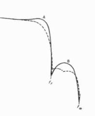
Fig. 19. Curves resulting from noise suppressor. Solid line represents initial measurement before correction, showing peak at A and return at B. Dotted line shows curve after applying corrective measures described.
