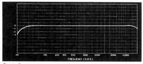
Fig. 2. Frequency response curve of audio amplifier at 30 watts output. Note that it is flat within less than one db from 30 to 20,000 cycles.
