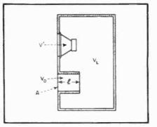
Fig. 1. Cross section through vented loudspeaker enclosure.
