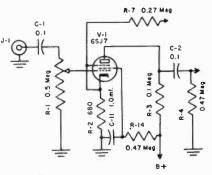
Fig. 5. Schematic of changes to circuit of V<sub>1</sub> when used as a pentode for increase of approximately 20 db in gain. Only required changes are in cathode resistor R<sub>2</sub> from 5,600 ohms to 680 ohms, and addition of R<sub>14</sub> and C<sub>11</sub>. No change is necessary in feedback resistor, R<sub>7</sub>.
