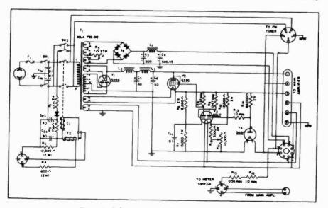
Fig. 28. Schematic of the power supply unit.
