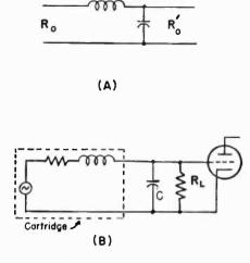
Fig. 1. (A) Conventional L-section low-pass filter configuration. (B) Circuit of magnetic pickup shunted by capacitor C and terminated by resistor R<sub>L</sub>, feeding grid of amplifier tube.
