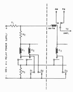
Fig. 2. Basic schematic of self-holding and automatic releasing relay circuits for station selectors.
