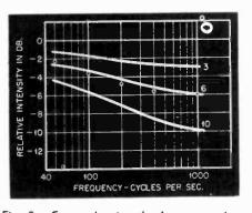
Fig. 2. Curves showing the frequency characteristic of each network section at various intensity levels.
