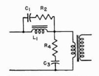
Fig.16. Simplified circuit of the phonograph equalizer.
