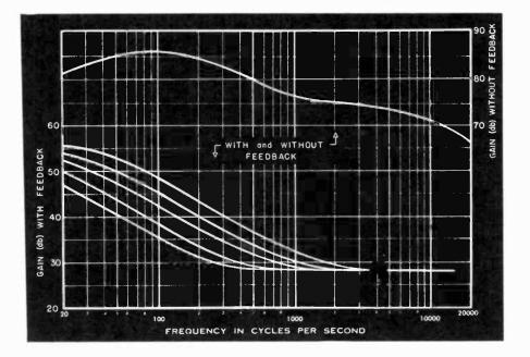
Fig. I. Response curves of preamplifier with and without feedback.
