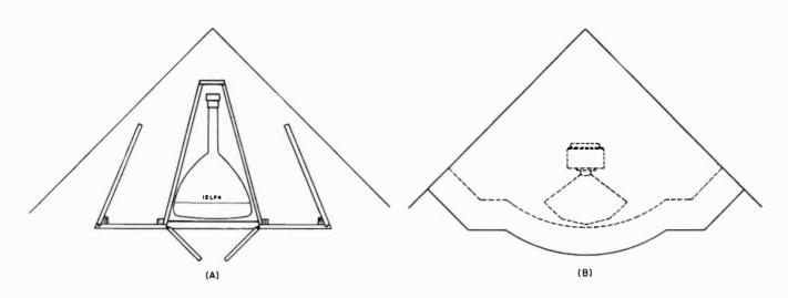
Fig. 4. (A) Cross section of the cabinet at the plane of the center of the picture tube to show location of tube enclosure. (B) Plan of the top (solid lines) and of the superstructure (dotted lines).
