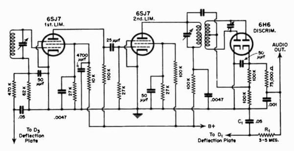
Fig. 2. Limiter and discriminator stages of typical FM tuner.
