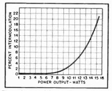
Fig. 7. Intermodulation distortion curve plotted against power output.
