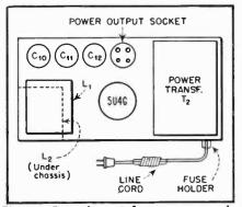
Fig. 5. Parts layout for power supply.
