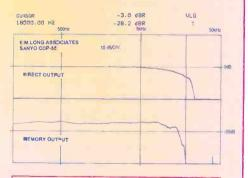
Fig. 8—Spectrum of output for recorded test pulse from Sanyo CDP-55, direct (top) and via memory (bottom).
