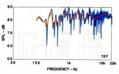
Fig. 8—Satellite 3-meter room response.
