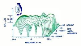
Fig. 5—Satellite vērtičal off-axis frequency responses.
