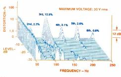
Fig. 11—Harmonic distortion for E<sub>1</sub> (41.2 Hz).
