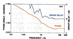
Fig. 2—Satellite phase response and group delay.
