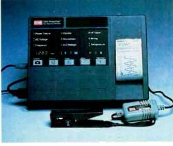
BMI PowerVisa 100G portable power-line monitor, used in six test sites.
