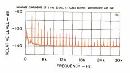
Fig. 4—Spectrum analysis of 1-kHz signal at rated output.
