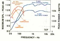
Fig. 13—Maximum peak input power and sound output.
