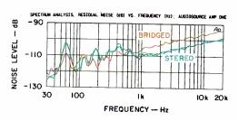
Fig. 7—Spectrum analysis of residual noise.
