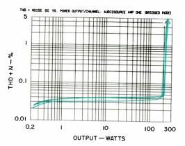
Fig. 6-THD + N vs. power output in bridged mode for three test frequencies; bottom curve is for 20 kHz.
