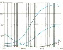
Computer analysis of Harmonic Time Alignment for four amplifier designs: 1) typical early solid-state, 2) typical recent solid-state, 3) typical tube, and 4) Nakamichi HTA.
