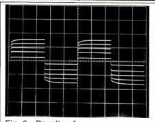
Fig. 6-Results of deliberate high-frequency overload from 1-kHz square waves at four different input levels. Note the symmetrical clipping; see text. (Scales: Vertical, 2 V/div.: horizontal, 200 µS/div.)
