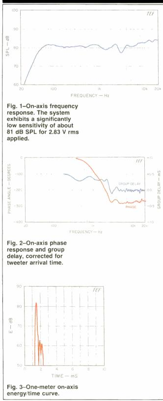
deviation of approximately  $\pm 3 \text{ dB}$  from 47 Hz to 20 kHz; its major feature is a 5-dB peak-dip combination in the crossover range of 2 to 4 kHz. If the crossover anomaly is excluded, the response is even tighter:  $\pm 2 \text{ dB}$  from 55 Hz to 10 kHz.
