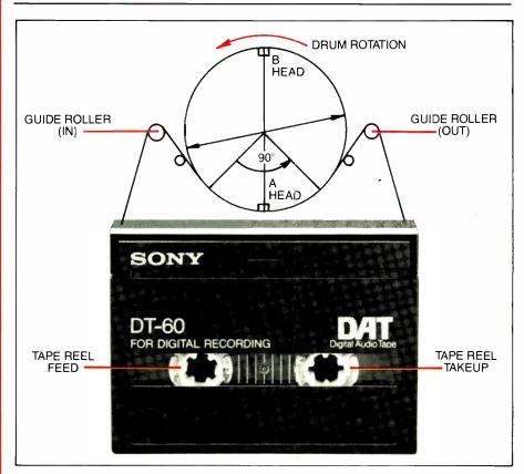
In the DAT format, digital data is recorded via a pair of magnetic heads mounted on a rotary drum that spins counter-clockwise at a rate of almost 2,000 RPM . . . This allows up to 2 hours of 16 bit digital music to be stored on a cassette only 3/3 the size of conventional audio cassettes.
