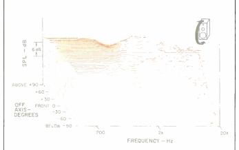
Fig. 5–Vertical off-axis frequency response, taken from below, up the front, and to the top of the speaker and normalized to the on-axis response.
