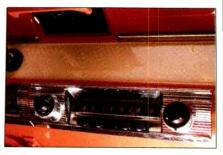
... or is it? Note the CD changer's remote control under the ashtray (top), the preamp knobs peeking out from under the radio buttons, and the digital display barely visible between 8 and 10 on the radio dial.
