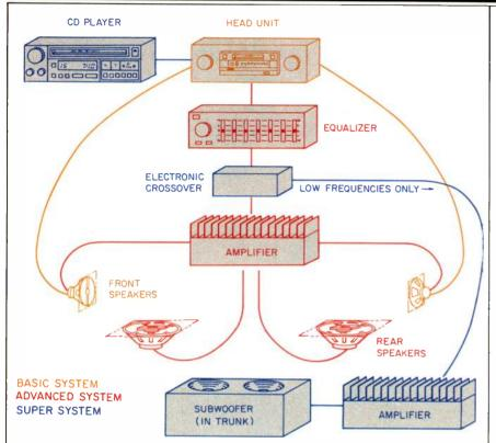
Fig. 1—In basic car-stereo systems, the head unit (tape and tuner sections) in the dashboard drives the speakers directly. In more advanced systems, separate amplifiers are used, allowing higher power output; equalizers may be separate (as shown), be combined with amplifiers,
