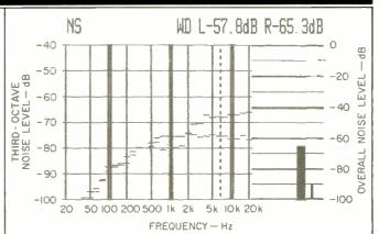
Fig. 7A—Tape S/N analysis, A-weighted, without noise reduction (upper trace and "L" readout at top) and with Dolby B NR (lower trace and "R" readout).
