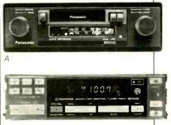
Stereo units with knobs at each end and the tape slot and tuning indicator jutting from the middle (A) fit the dashboard spaces in most older cars and many newer ones. The dashboard spaces in more and more new cars, however, are rectangular, DIN-standard slots for which flat-front units (B) are designed. Note the station indicators: Pointer-and-dial (A) vs. digital readout (B). The digital display panel of the unit shown here flips down for access to the cassette slot and subsidiary controls.
