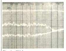
Fig. 2—FM frequency response (top trace), and separation for weak (middle trace) and strong (bottom trace) signals.
