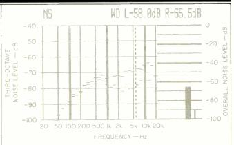
Fig. 7—Tape section S/N, A-weighted, without noise reduction (upper trace and "L" readout at top) and with Dolby B NR (lower trace and "R" readout).
