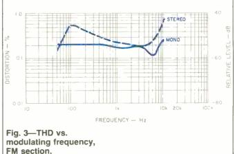
With strong-signal input, separation was 42 dB at 1 kHz and 100 Hz, and 32 dB at 10 kHz. These results are excellent.
