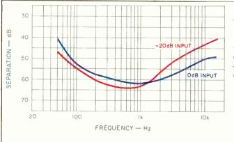
Fig. 7—Separation measured by the CBS Technology Center for an FMX decoder shows high mid-band separation at two signal levels.
