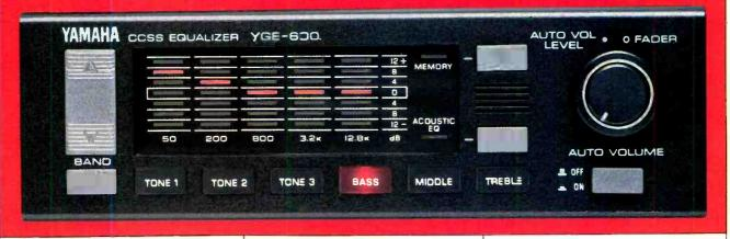
The Auto Volume circuit worked smoothly, especially once I had adjusted its front-panel setting. In my car, which is fairly noisy, the system worked best with the control nearly at its maximum. The automatic adjustment range is deliberately limited: Yamaha's instruction manual shows a level change of only 14 dB for a 20-dB change in ambient noise.
