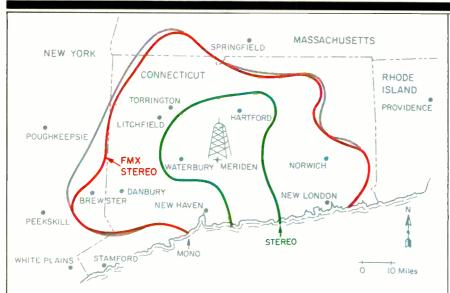
Fig. 1—Reception contours for a station using FMX, showing distance limits at which tuners could achieve 60-dB S/N in mono, FMX stereo, and conventional stereo. Note that quiet stereo reception with FMX extends nearly as far as quiet mono reception.
