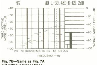
but without (upper trace and "L" readout) and with Dolby C NR (lower trace and "R" readout).
