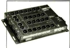
Complex equalizers should be set up by a competent installer, preferably with the aid of test instruments, and then left alone. Such equalizers are often mounted in the trunk to discourage fiddling.
