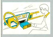
Fig. C1—To check on whether noise is being induced into the receiver, pull it from its mountings while it remains connected, and listen for a drop in noise level.
