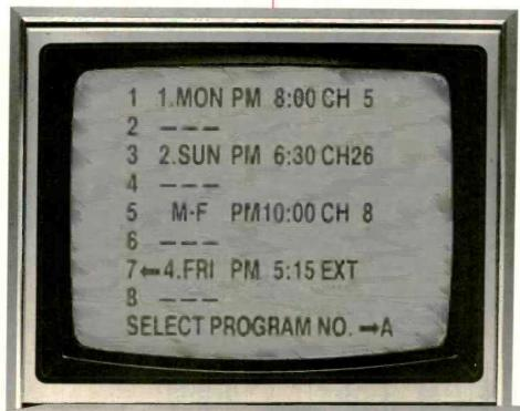
tures. In addition to incredible hi-fi sound and remote input capability, you get the flexibility of programming directly through the machine. Four heads provide picture-perfect record, playback and special effects. A cable-ready, 139-channel tuner provides 28-day/8 event programmability; a lighted tape area allows tape usage monitoring.
