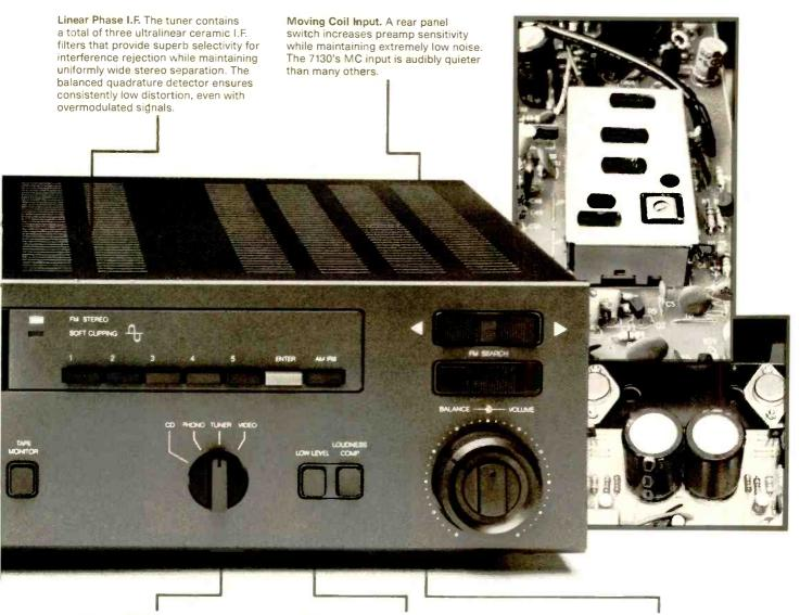
CD Input. The 7130 receiver has a separate CD input (not merely a renamed AUX input) for a Digital Compact Disc player. There is no input circuit that could be overloaded by high level peaks; the signal goes directly to the Volume control before it is amplified.
