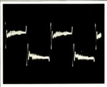
Fig. 2—Response to a 1-kHz square wave.
