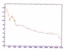
Fig. 6—Spectra of the opening 1.7 seconds from two versions of "Lux Aeterna" on the second Reference Recordings HDCD sampler. The purple curve is for the HDCD version, the orange curve for a version recorded through a conventional Sony 1630 16-bit A/D converter. Note the slight high-frequency rolloff in the HDCD spectrum, starting a little below 2 kHz.
