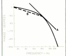
Fig 1—Phase response of an 8-pole Butterworth anti-aliasing filter. At any given frequency, group delay is represented by line A, which is tangent to the phase response, and phase delay by line B, which is between the origin and the phase response at that frequency.
