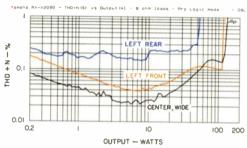
Fig. 12—THD + N vs. amplifier output,
