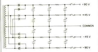
Fig. 2-Power-supply configuration. Four diodes at center form one bridge rectifier, top and
