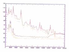
Fig. 9—Spectra for the "heads" (upper pair of curves) and "tails" (lower pair) of a high-treble piano note. The purple curves are for the HDCD-encoded version, the orange curves for an unprocessed 16-bit recording of the same event.
