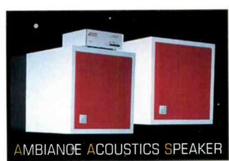
nstead of a woofer. tweeter, and crossover, the California Cube. from Ambiance Acoustics, uses four full-range 41/2-inch drivers plus an external equalizer. This equalizer features a 64-Hz bass rolloff filter with an 18-dB/octave slope, an EQ bypass switch, and a tape monitor. An optional "purist" upgrade replaces
