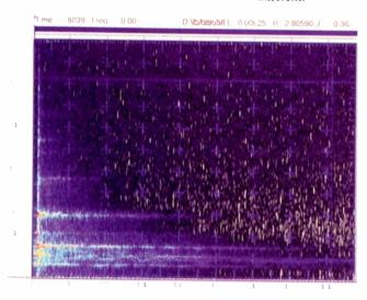
Fig. 10—"Three-dimensional" spectrogram of the unprocessed 16-bit recording of the entire piano note depicted in Fig. 9.
