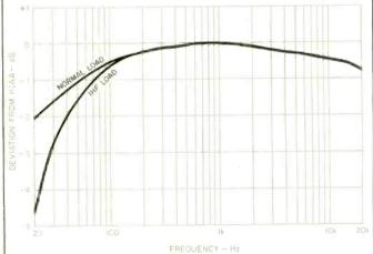
Fig. 3—RIAA equalization error for normal load (90 kilohms and 250 pF) and IHF load (10 kilohms and
