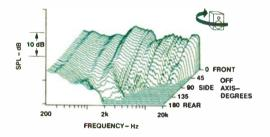
Fig. 3—Horizontal off-axis frequency responses.
