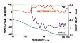
Fig. 2—On-axis phase response, group delay, and waveform phase (see text).
