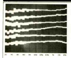
Fig. 2—Forward and "reverse" record/playback responses, overlaid. From top to bottom: EXII tape without NR, EXII with Dolby C NR, SX tape
