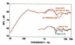
Fig. 1—On-axis frequency response.
