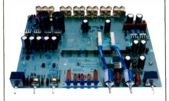
By gold plating all input and output jacks, and then directly mounting all jacks, switches, potentiometers and other laboratory grade components on a double copper-plated, glass epoxy printed circuit board, signal losses and noise are dramatically reduced.
