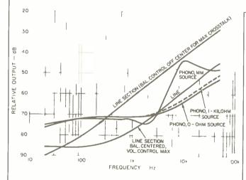
Fig. 6—Crosstalk vs. frequency for line and phono sections. Note increase in line-section crosstalk when balance control is moved towards driven channel. (The same effect was seen
