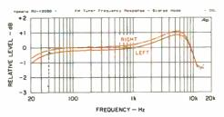
Fig. 8—Frequency response and channel balance, FM tuner section.
