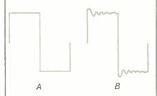
Fig. 2—Square wave before (A) and after (B) phase shift.
