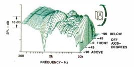
Fig. 4—Vertical off-axis frequency responses.
