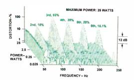
Fig. 7—Harmonic distortion for E<sub>1</sub> (41.2 Hz).
