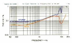
Fig. 9—THD + N vs. frequency, FM tuner section.
