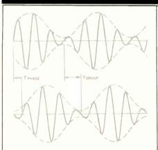
Fig. 3—Envelope distortion: Where phase shift is nonlinear, different phase-delay and group-delay times cause unequal delay of the carrier and modulating signal, changing the relationship between them.
