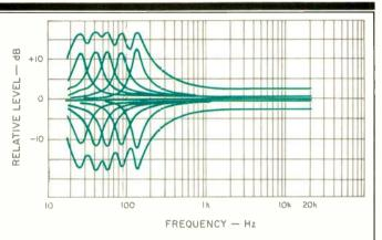
Fig. 1—Swept-frequency responses of each filter section at maximum boost and maximum cut,
