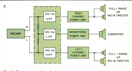
Fig. 1—System connections for center-channel woofer, using monophonic amplifier (A) or stereo amplifier (B) for center channel.
