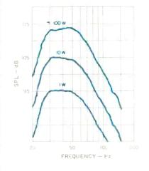
Fig. 6—Power compression of project subwoofer. Note lack of compression at levels below 10 watts, slight compression above.
