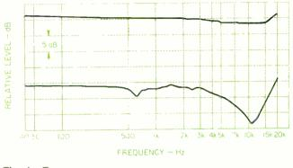
Fig. 1—Frequency response and separation.
