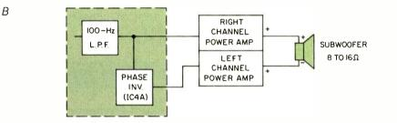
uses a monophonic power amplifier to drive the center-channel subwoofer. If you do not have a suitable mono power amplifier, no problem; Fig. 1B shows how to connect a conventional stereo power amplifier to drive the center woofer. A built-in phase inverter drives one channel of the stereo power amp, so the subwoofer can be differentially connected across the R and L output terminals to use the power of both amplifier channels.
