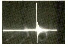
Fig. 5— Two-tone phase test (2 kHz in one channel, 20 kHz in the other; see text).
