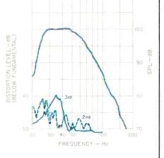
Fig. 7—Distortion at 100 dB drive level. Levels shown for second- and third-harmonic products have been shifted up by 20 dB to fit chart recorder.
