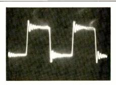
Fig. 4— Single-pulse test; note ringing.
