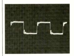
Fig. 2—Response to a 1-kHz square wave.
