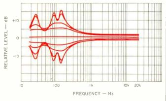
Fig. 2—Swept-frequency responses with 31.5-, 90- and 125-Hz filters set
