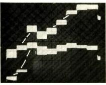
Fig. 6—One-third octave response of stagemonitor loudspeaker before (top curve) and after (bottom curve) equalization. Vertical sensitivity, 5 dB/div.; horizontal, 1/3 octave from 25 to 250 Hz. nection with a preamp/receiver and a tape recorder. There are also stereo outputs for both low and high frequencies from the electronic crossover. The monophonic warble tone is fed through left and right outputs. The microphone input is also a phono jack.
