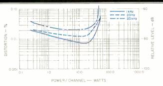
Fig. 1—Power output vs. THD.
