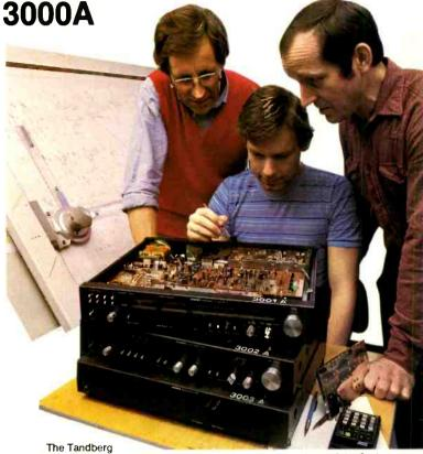
TPT 3001A Programmable FM Tuner, like all the other members of the Series 3000A, features discrete components — not integrated circuits — individually selected to meet ideal performance parameters.
