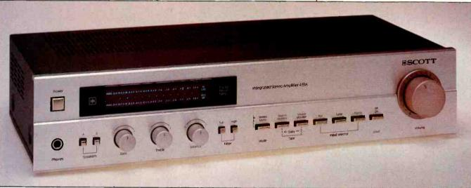
H. H. Scott's 438A integrated amplifier includes many of the features of Scott's top-of-the-line models. Among them are dual fluorescent auto-range peak-hold power meters, two tape monitor functions, a d.c.-configured output-capacitorless power amplifier stage, loudness contour, electronic circuit protection, subsonic and high-cut filters, plus conventional bass and treble controls.
