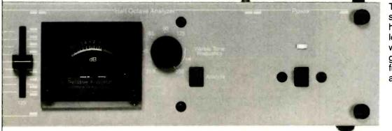
The analyzer section features a highly damped level meter and a warble-tone generator whose frequency is adjustable.
