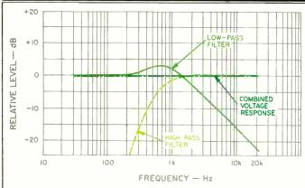
Fig. 4—Responses of the low- and high-pass filters,
