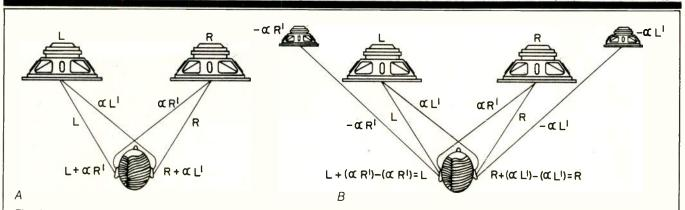
Fig. 2—In a normal speaker setup, each ear hears both speakers (A), while in the image recovery system, the left ear hears only the left speaker and the right ear only the right (B). See text.
