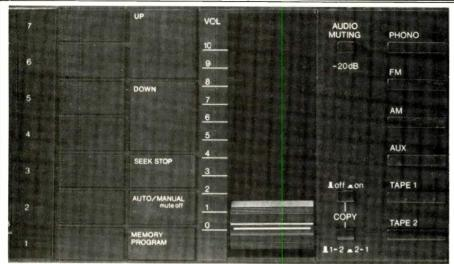
Neat and knobless main control section of the R-851 concentrates tuning functions (including seven presets each for AM and FM) to the left, general audio functions at the right. Hinged lower flap conceals tone controls, speaker selector, MM/MC phono selector, and other miscellaneous controls.
