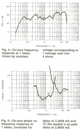
1 meter, corrected for (M) the midrange's air-path
