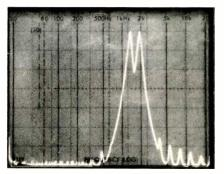
Fig. 8—Range of variable-turnover bass and treble tone controls.
