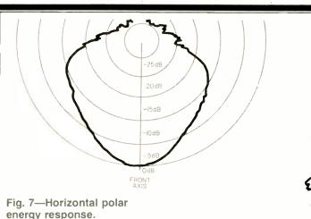
point to the listening position. The lower measurement corresponds to a traditional, 30° off-axis, left-channel stereo speaker location. Since the response is more uniform in the straight-ahead position, I recommend rotating these speakers toward the normal listening position.
