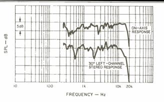
Fig. 6---Three-meter room response.
