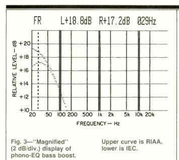
of 1.6 dB. The 0.1 dB difference is attributable to measurement equipment tolerances.
