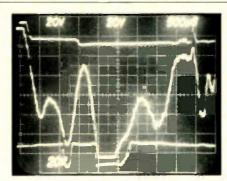
large signal voltage swings, Class-H circuitry of Soundcraftsmen RA7502 power amplifler.
