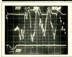
Figs. 1A and 1B— Multiple traces showing how B+ (Fig. 1A) and B-(Fig. 1B) voltages adjust themselves in anticipation of
