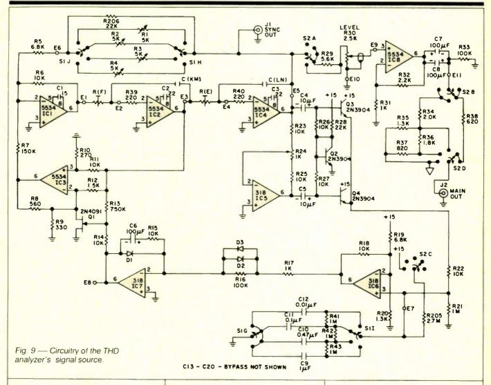
octave low-pass characteristic. Notice that the phase of this output lags that of the bandpass output by 90 degrees at all frequencies. This feature is used to provide the required 90-degree phaseshifted fundamental signal to the frequency detector in the auto-tune circuit.
