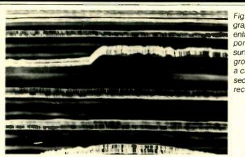
Fig.5 — Photomicrograph at about 35X enlargement of a portion of the record surface showing the groove geometry of a cannon shot section of the recording.
