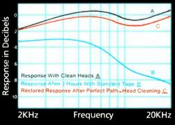
Playback accuracy of a calibrated test tape. Note that after only three hours' play, high frequency response is reduced by as much as 10 dB. One cleaning with the Perfect Path Head Cleaner restores the highs to within 1 dB of the original response.
