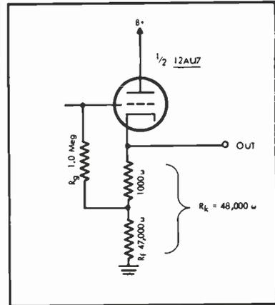
Fig. 17. Typical cathode-follower circuit. been equal to  $A$ , namely 0.95, and  $Z$  would have been 20 megohms.
