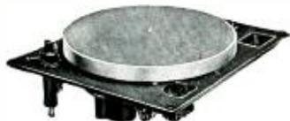
The hush of an empty church, even though the synchronous motor is running—this is the Connoisseur, crafted in traditional English quality. Precision machining assures pure sound reproduction. Non-magnetic, 12" lathe-turned table; precision ground spindle; phosphor bronze turntable bearing;  $\pm 2\%$  variation provided for all 3 speeds; hysteresis motor. **\$110.00**
