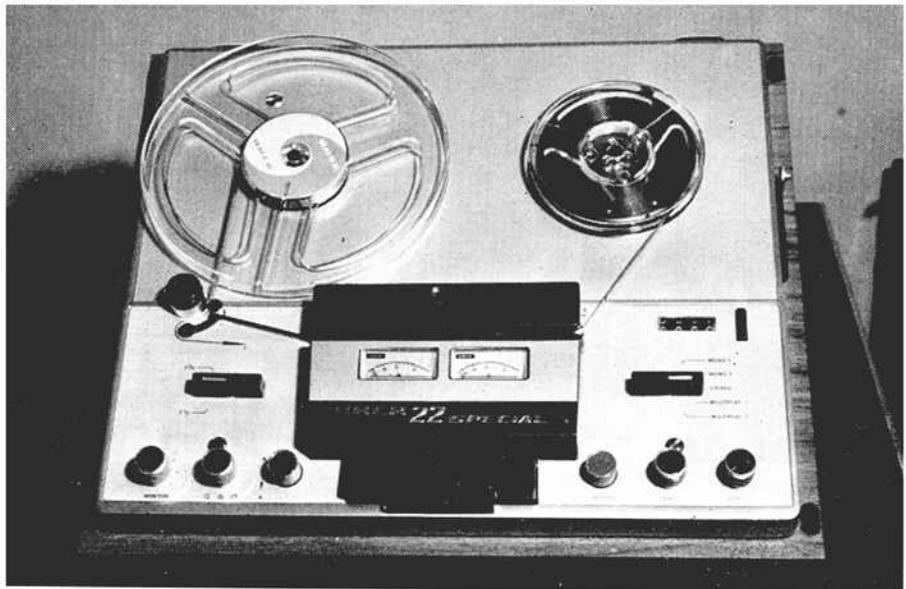
Fig. 5. Top view of the recorder with plastic cover removed.
