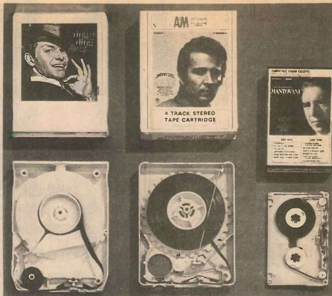
cassette (Philips) showing relative size and intricacy. Cartridges employ endless loops of lubricated 1/4" wide tape in reel-to-reel format. Ampex produces an extensive selection of
