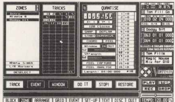
The Zone Page offers complex conditional processing of tracks. Here the quantize facility is ready to operate on the chosen tracks.
