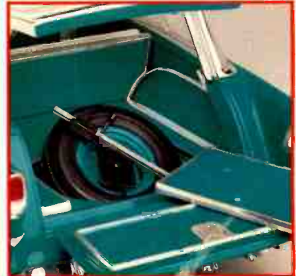
The two-piece tailgate opens to reveal the spare tire compartment, complete with spare tire and jack.
