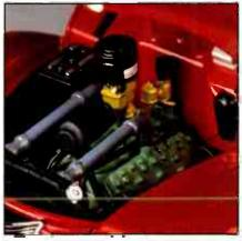
Raise the hood to examine an authentic miniature of the 85 hp, 221 cubic inch V-8 engine.
