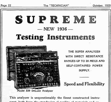
ment, both from the standpoint of quality of materials and engineering skill. The 339 DeLuxe virtually spreads the entire circuit of the set out on your analyzer panel like a diagram. It is a combination point-to-point tester and analyzer, providing a complete resistance, voltage and current analysis and tube testing direct from the radio socket, including the metal tubes.
