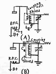
Fig. 23-1—An open circuit in either the coupling-coil circuit shown in (A), or in the coupling-condenser circuit shown in (B) will cause lack of sensitivity in an r-f or i-f amplifier which employs them. These obscure troubles would not be revealed by the usual voltage-current or resistance analysis of the receiver.
