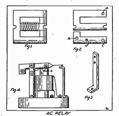
shown in Fig. 2. Holes are drilled at a, b, and c, Fig. 2, to hold the transformer iron together.
