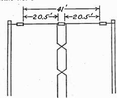
This sketch shows an insulator inserted in the center and each leg of the lead-in connected to one-half of the aerial. However the lead-in can be connected to either end but in this case only one leg is connected and the other is dead ended.
