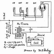
were put in series, and the 84 tube and resistor R<sub>1</sub> in parallel with them so they would take 1.75 amperes: 2A7 in series with that combination with resistor R<sub>1</sub> in parallel with the 2A7 so that it will take 1.75 amperes. The 2A5 is put in series with the rest of them. The total current taken by the tube filaments is 1.75 amperes.
