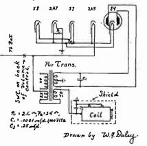
were put in series, and the 84 tube and resistor R<sub>1</sub> in parallel with them so they would take 1.75 amperes: 2A7 in series with that combination with resistor R, in parallel with the 2A7 so that it will take 1.75 amperes. The 2A5 is put in series with the rest of them. The total current taken by the tube filaments is 1.75 amperes.
