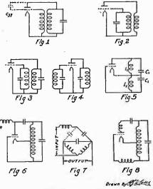
On shorter wavelengths, however, the electrostatic couplings between the coils and the tube elements become very important and at very high frequencies may exceed the magnetic coupling. Care must therefore, be taken in the layout for high frequencies as the capacitive and inductive couplings are usually of opposite sign.
