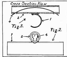
First drill a three-sixteenth inch hole 1/4 inch in from each end of the piece of tubing and smooth the edges of the holes. Part 2 shown in Figures 1 and 2 is then formed. Next grind each edge of the piece of spring back from each end about 1/8 inch to form a tab 1/8 inch wide as shown at 4 in Figure 2. Be very careful, however, not to get the spring hot while grinding as this will draw the temper of the spring and ruin it.
