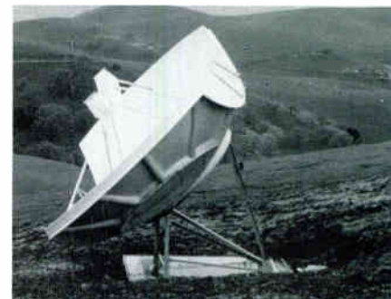
The Simulsat earth station from Antenna Technology.
