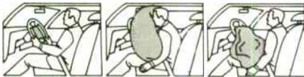
In a serious crash the air bag automatically inflates in less than 1/25 of a second, protects and then deflates.
