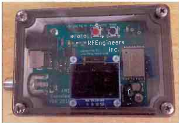
The Watch Dog (WD1) is a professional AM / FM / NOAA Weather receiver. It has user definable alarm states. The WD1 tracks RSS, SNR, Audio, RDS, Pilot and NOAA 1050Hz for presence/validity. It can be programmed using a Windows program, which is available.
