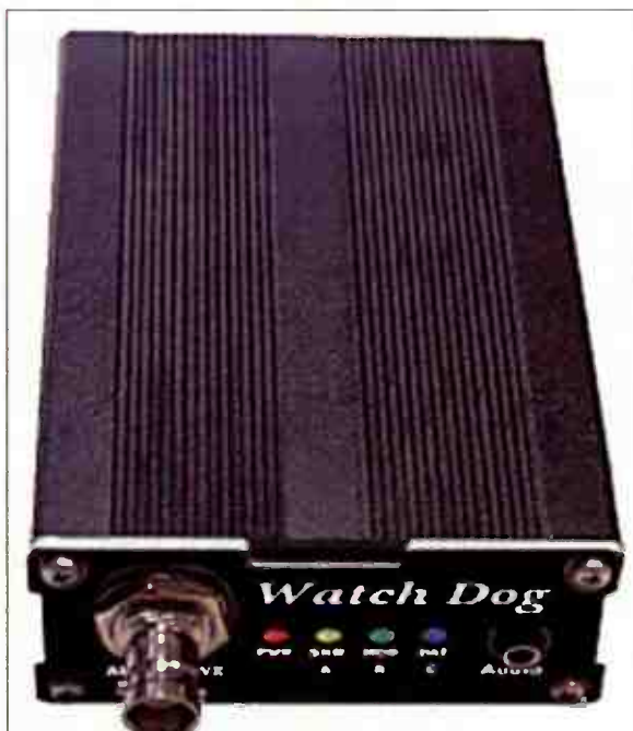
The Watch Dog (WD1) is a professional AM / FM / NOAA Weather receiver. It has user definable alarm states. The WD1 tracks RSS, SNR, Audio, RDS, Pilot and NOAA 1050Hz for presence/validity. It can be programmed using a Windows program, which is available.
