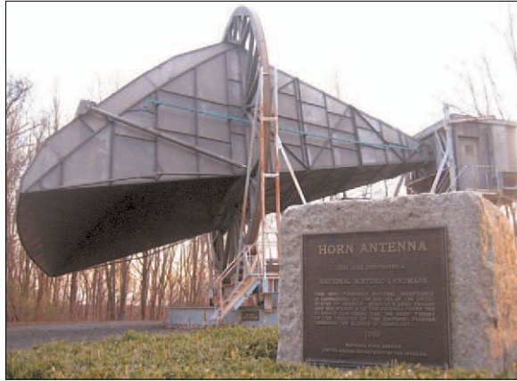
Bell Laboratories horn antenna. This antenna was built for the purpose of using the Echo satellites for communication relays. Later it was used in the discovery of cosmic background.
