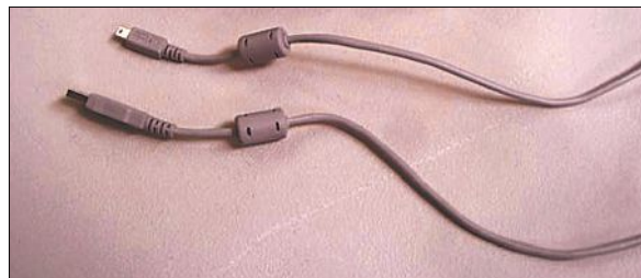
Computer and camera cables often have ferrites to keep signals clean.
