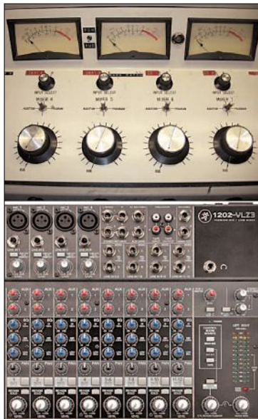
Simple Air console above, complex Production console below.
