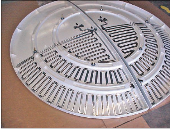
Zig Zag Heater Tape Applied
