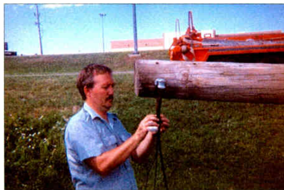
Dave Dunsmoor is shown rigging the dipole antenna.
