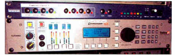
The Tieline can be fed by any station, using the BTI switcher.
