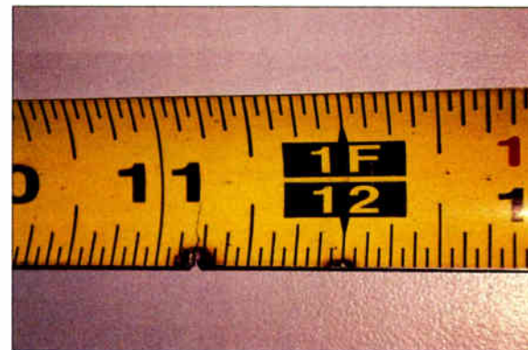
Waving a metal tape around under a tower may result in more than a measurement of distance.
