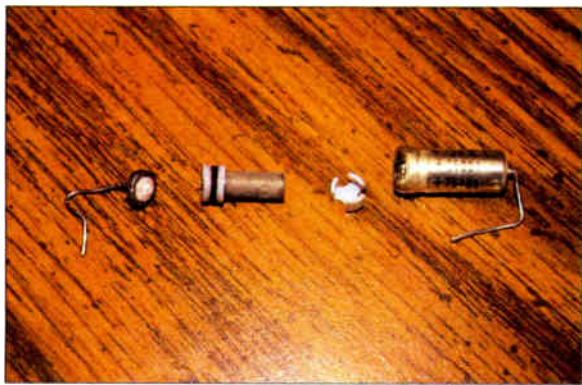
A backwards capacitor in an energized circuit is not exactly something you should want to touch.
