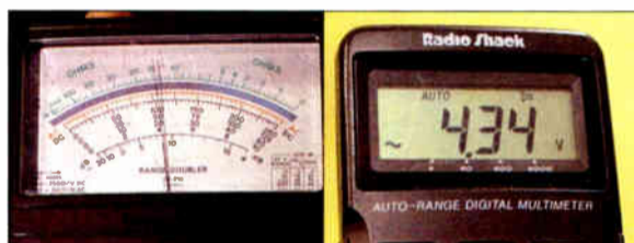
A typical VOM shows a little over 4.2 V AC.
