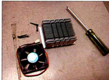
Buy a ball-bearing type fan and use only the fan in the replacement process.
