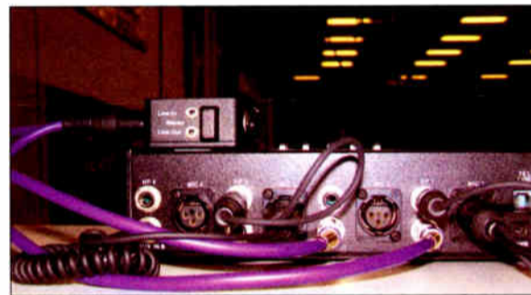
The Daptor Three has both balanced XLR and unbalanced 3.5 mm stereo inputs.
