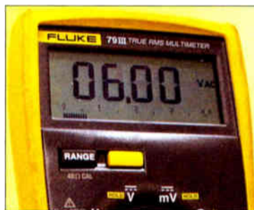
A true RMS DMM gets the correct reading.
