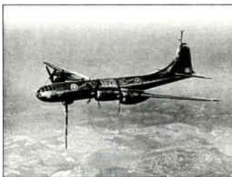
The Stratovision transmission system.
