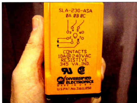
The Diversified Phase Loss Relay.
