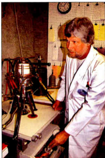
By carburizing the filament, tube life is significantly enhanced.
