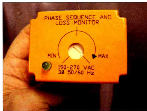
The top of the Phase Loss module. Note the adjustable trip point.
