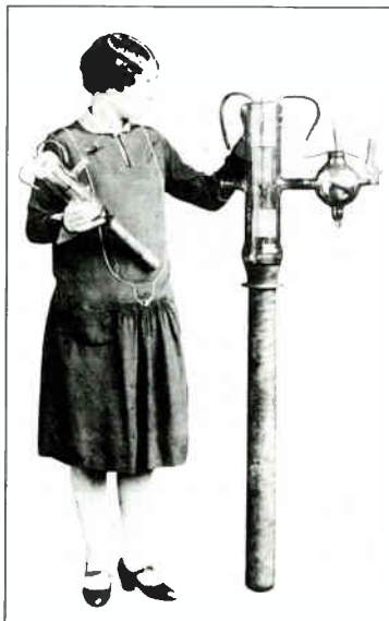
Power tubes like the 207 and the 862 gave broadcasters a much "bigger voice."
