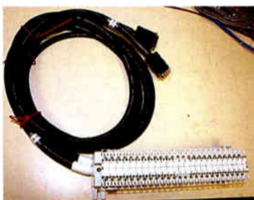
A typical factory-built pre-wire using a Krone block.
