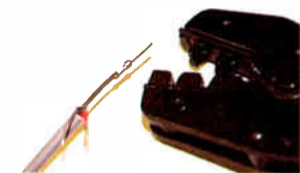
A pin properly crimped to the wire.
