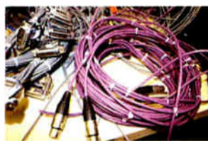
Using Belden 1800B cable, the bulk adds up fast.
