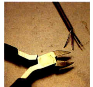
Strip the wire, twist to bring wires together, then clip the insulation back 1/16 inch.
