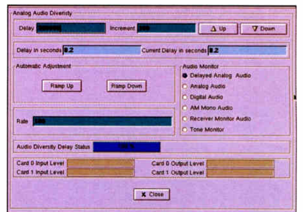
The analog delay (diversity) screen.
