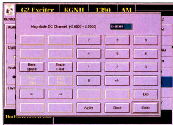
Magnitude DC Offset adjustment screen.
