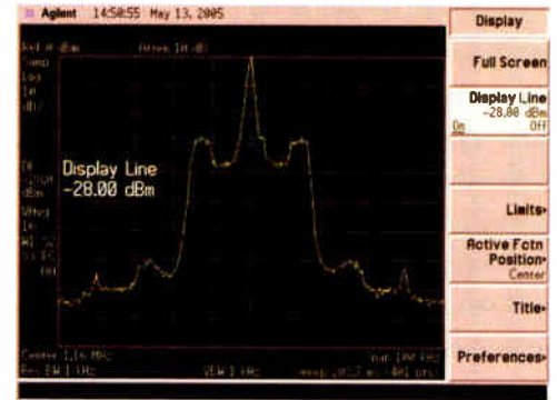
Figure 4 - Station #1, single tower, good bandwidth.
