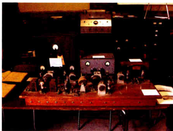
Early Armstrong broadcasted oscillator and balanced modulator (foreground), with early FM receivers.
